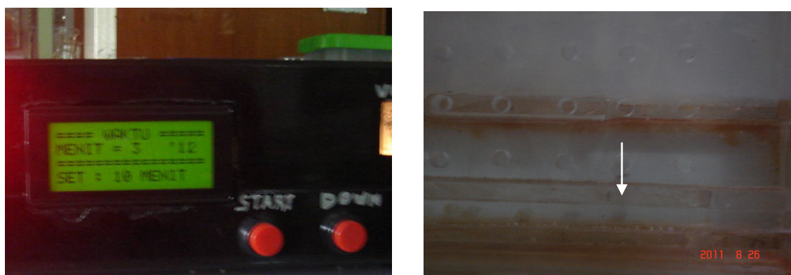
Figure 5. The performance of electrophoresis instrument design (The air bubbles was marked by white arrow).
